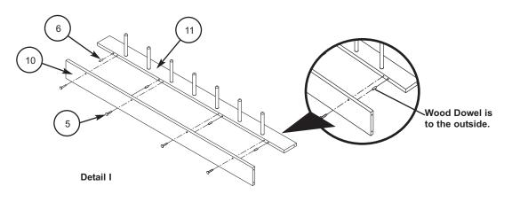
Attach the Lower Base Support Assembly and one Neck Support to the End Panels (#2) using eight Hex Socket Lag Screws (#5) per side. (Detail J).
